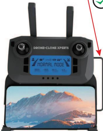
**IMPORTANT NOTE:** The connector at the **bottom** of the remote is **only used for charging the remote control**. it is **NOT** for image transmission connection data.
