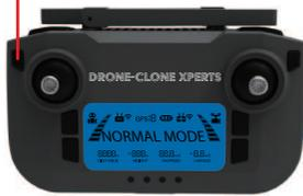
**NORMAL MODE:** Low speed with stable flight. Obstacle Avoidance function **ENABLED** in this mode.
