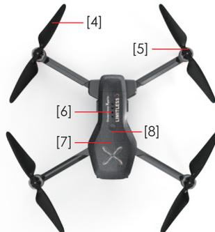
[4] Propeller Blade [5] Motor [6] Power Indicator
