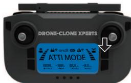
Press and hold the “headless mode” key for 5 seconds. The remote control will make a “BEEP” sound, indicating that GPS function is turned OFF. This will allow take-off while in ATTI MODE.
