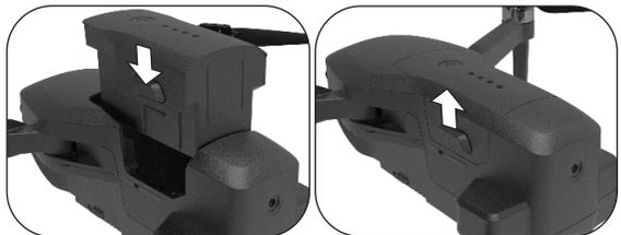
**⚠ REMINDER:** If the battery is not installed properly, it is likely to cause an interruption in power, which can lead to major accidents. After the drone is used, please turn off battery power and remove it from the drone. Store the battery in a cool / dry place to prevent battery damage from the heat emanating from the drone's motors after flight.
