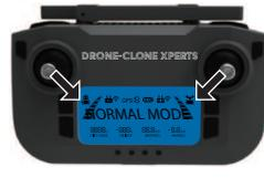
When the throttle joystick & the directional joystick are pushed to the lower left corner and lower right corner at the same time (Figure 1), or pushed to the lower right corner and lower left corner at the same time (Figure 2), the drone will become unlocked & you'll notice the motors/propellers will start spinning in preparation for takeoff. The drone will remain on the ground during this time...until the left joystick is pushed forward, which will then cause the drone to take flight
