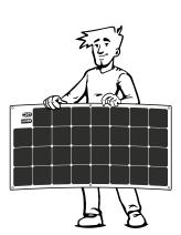
The panel can be supported by the edge but only by keeping it vertical and without exerting excessive pressure on the cells. The panels should not be gripped by the ends and
