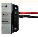
Connect cable B to the charge controller (BAT +/-) respecting the polarities.
