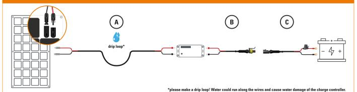
Remove the caps from the monopole Junction Box and connect the MC4 connectors of cable A (see image above).
