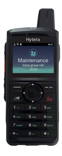
The PNC380S is a compact, rugged, and easy-to-operate Push-to-Talk over Cellular (PoC) and Wi-Fi device. The PNC380S supports nationwide voice and video group calling, dispatching, and GPS location tracking It is AT&T Network Ready, has T-Mobile IoT Network Certification, PTCRB certified and features an optional dash-mount car kit.
