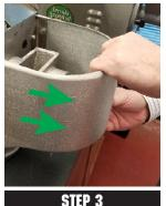
Remove the front cover by gripping the cover and pulling away from the grinder.
