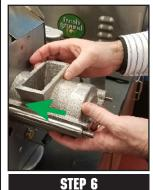
Place the **Front Cap** on guide rods as shown below.
