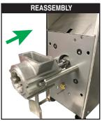
Slide **Auger Housing** onto the guide rods until flush with front face of machine.
