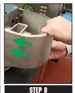
Place the front cover on machine. (magnets will hold front cover on)
