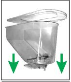
Place Chute on top of Auger Housing, confirm it is seated securely.
