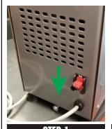
Turn the machine to the off position. (down)
