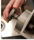
Pull the **Rotary Plate** and **Auger** out of **Auger** Housing.
