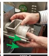
Place hand on the back of the **Auger Housing** and pull forward removing the entire **Auger Assembly**.
