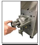
Holding the Rotary Plate, insert into Auger Housing and rotate until seated firmly.
