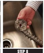
Hold **Auger** with a cloth for firm grip and unscrew **Rotary Plate**.
