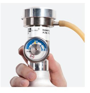
B. Attach demand regulator to calibration gas cylinder, and connect one end of tubing to the regulator.
