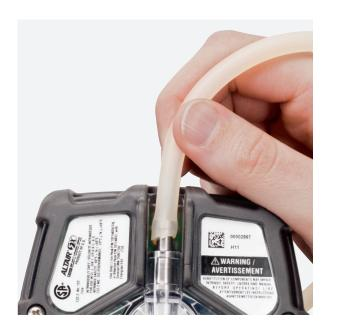
**C.** Connect other end of tubing to pump inlet.
