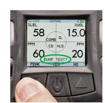
**A.** From measure screen, press ▼ button to display BUMP TEST?
