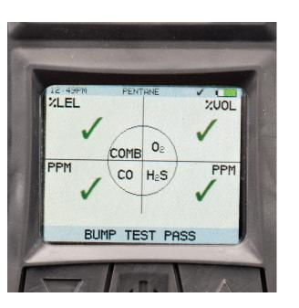
**B.** BUMP TEST PASS indicates successful sensor bump test. Next sensor displays and process repeats. BUMP TEST FAIL displays any sensor that failed bump test.
