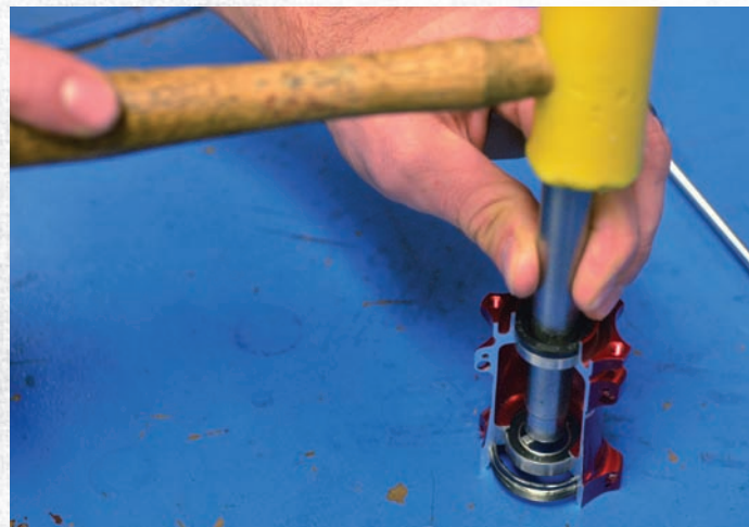
7 Using a punch, the woodruff key and a mallet, tap the drive side bearing from the hub shell.
