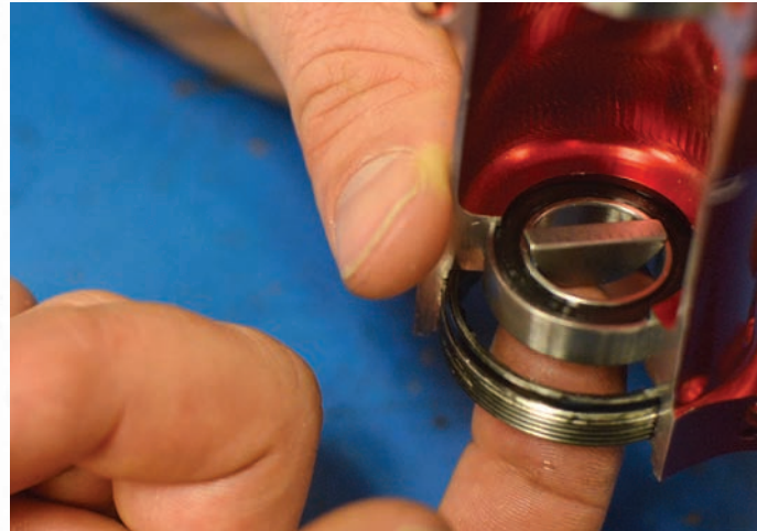
6 Install the woodruff key (on the drive side first) by inserting the key through the bearing with a finger or needle nose pliers.
