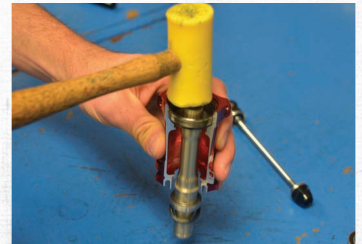
9 Using a plastic mallet, tap the axle to remove the non-drive side bearing.
