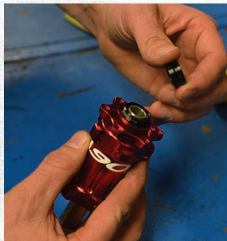
3 Remove non-drive side end cap by hand. Unthread the preload adjuster nut using a 20mm Cone Wrench. (Note: This is a reverse thread. Turn the adjuster in the “-” direction.)
