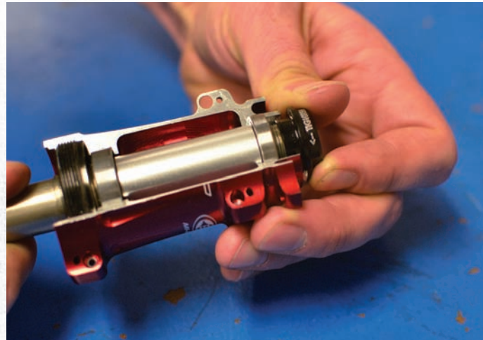
16 Thread the NEW axle nut (with seal) onto the axle. Make sure the wrench flats are on the outside.
