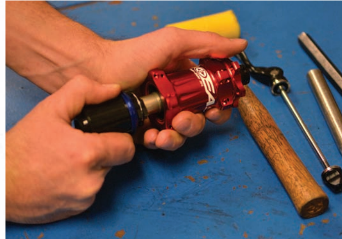
2 Pull the cassette body from hub shell.
