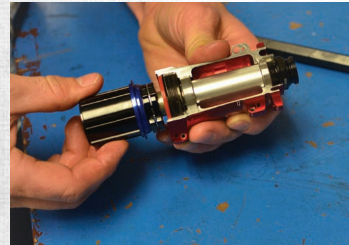
20 Re-install the cassette body by pushing gently and turning counterclockwise (to prevent the pawls from cutting the red seal).
