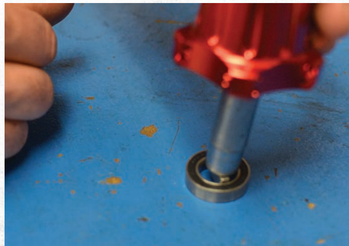
7 Using a punch, the woodruff key and a mallet, tap the drive side bearing from the hub shell.
