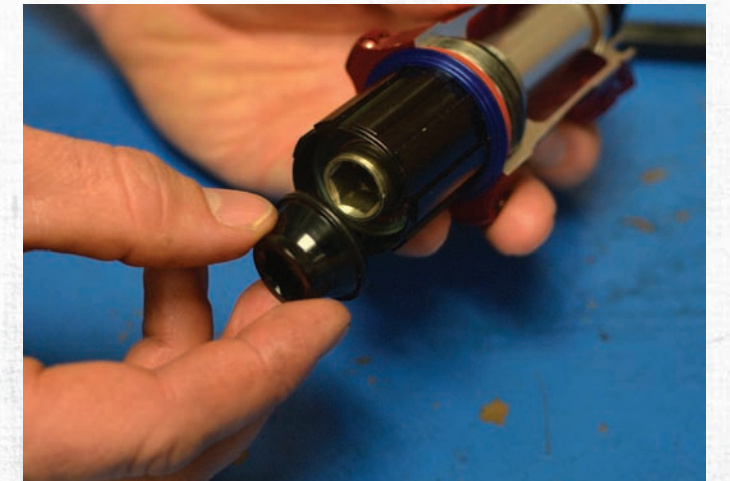
21 Re-install drive side end cap by pushing gently.
