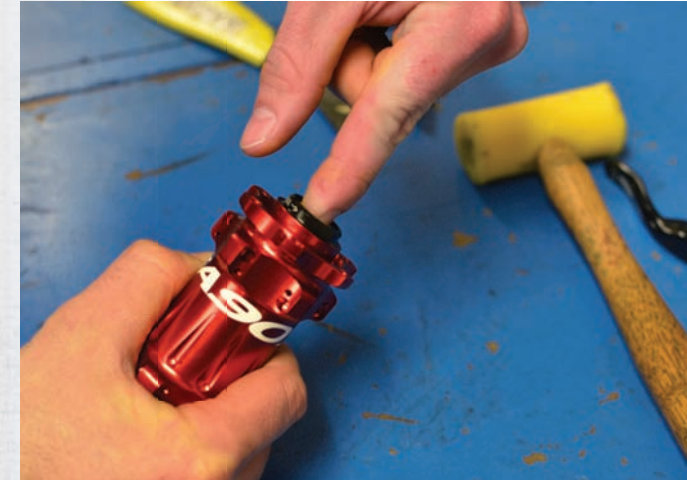
4 Push the axle away from the preload adjuster and remove the adjuster.
