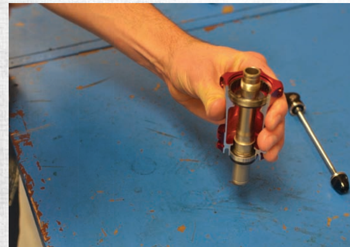
9 Using a plastic mallet, tap the axle to remove the non-drive side bearing.
