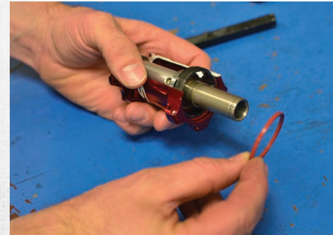
19 Add a coat of Easton Cassette Body Grease to the drive ring. Re-install (with lip facing out) the red cassette body seal.
