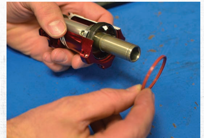
5 Remove the axle. Using a finger nail or a dental tool, remove the red cassette body seal.
