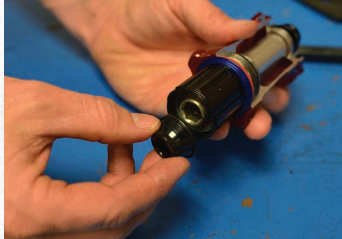
1 Remove drive side end cap.
