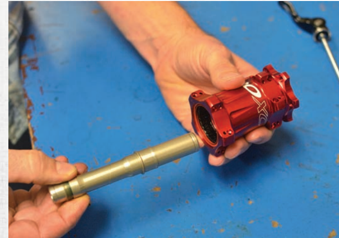
8 Install the axle backwards so that the drive side of the axle sits against the non drive side bearing.
