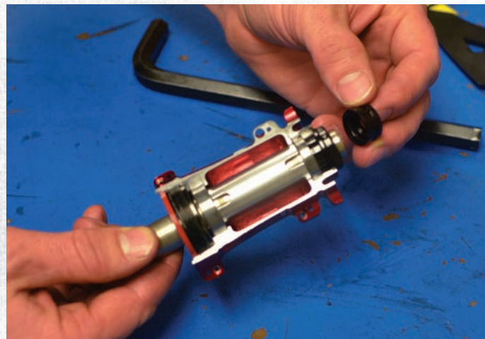
18 Push the non-drive end cap onto the axle.
