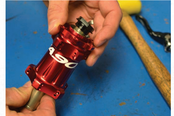
4 Push the axle away from the preload adjuster and remove the adjuster.
