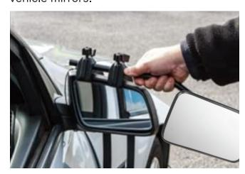
Tighten the wing knob thumb screws to firmly secure them in place.
