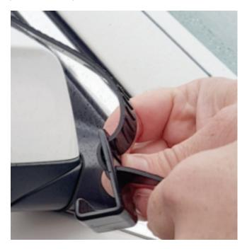
Place the protection pads onto the ends of the wing knob thumb screws and push to secure them in place.
