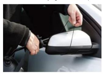
Position the clips onto the rims of your vehicle mirrors.
