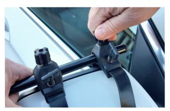
Wrap the straps around the back of your vehicle mirrors and fasten the clips to the rims of your vehicle mirrors.
