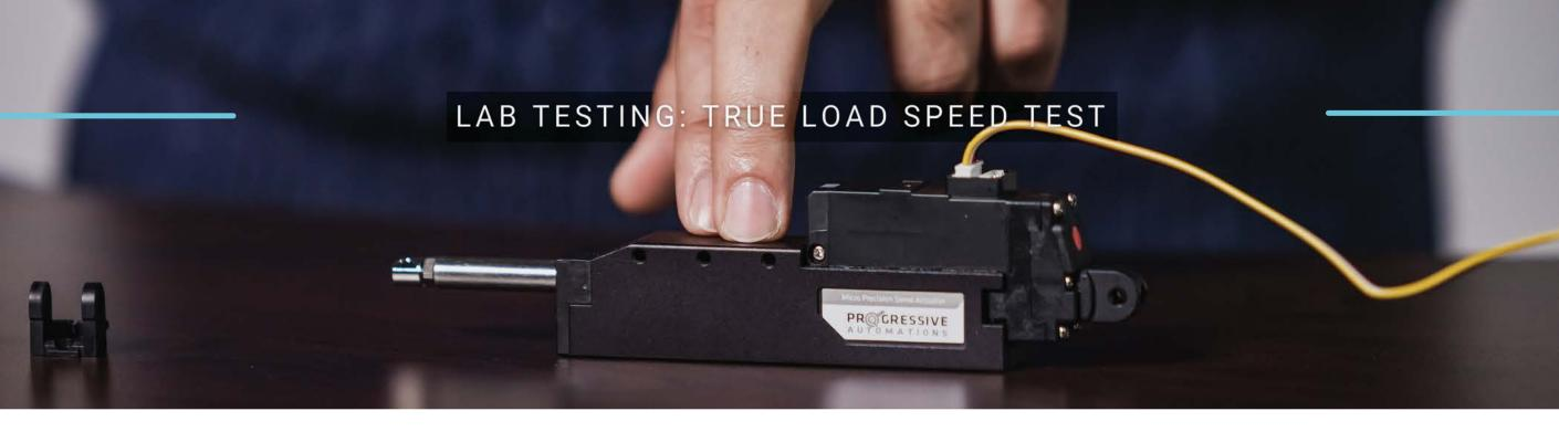
Once bench testing of the linear actuator has been completed, it is time to test it under load. The load should match what will be expected when in the desired application. The bench test methods are all applicable to the lab tests, with a few additions.
