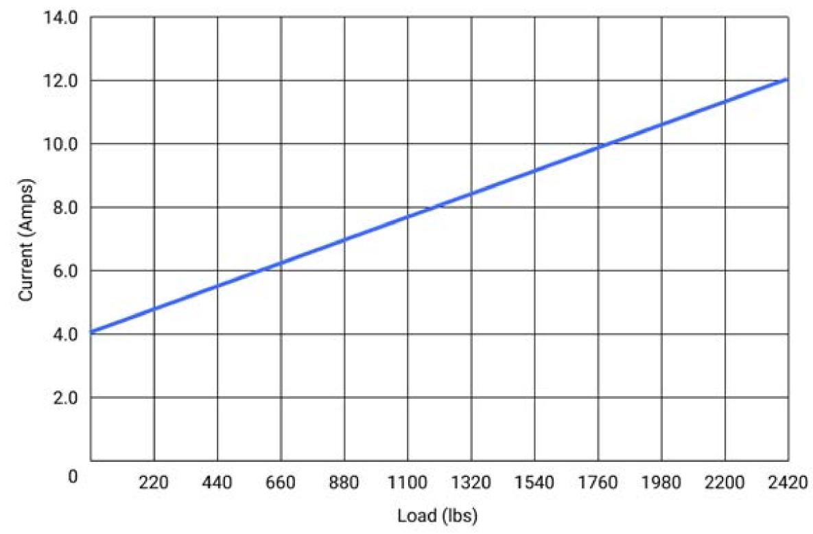
Since the linear actuator is now under load, the speed will decrease, and the actuator will draw more current. Knowing the current draw of the linear actuator under load will help select an appropriate power supply. To measure the current draw of the linear actuator under load, use a multimeter, as in the bench test.
