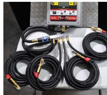
Completed 4-hose manifold assembly.
