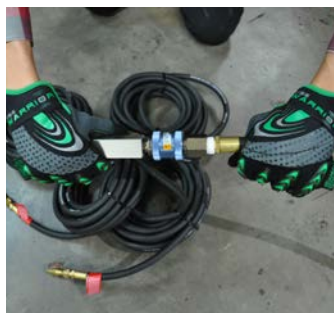
Step 4. Connect the other end of outlet hose to the air pressure release valve.
