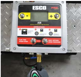
Step 3. Connect 1/2" outlet hose assembly directly to inflator air outlet.
