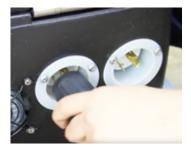
drainable location. Activate the pump-out switch on the front of the machine and open the ball valve on the pump-out connection. The Breeze<sup>™</sup> will automatically drain recovered water from the tank.
