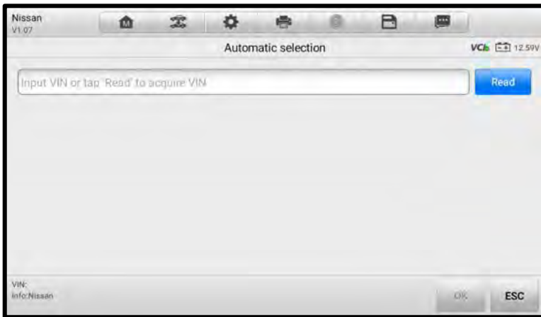
Figure 4-8 Automatic Selection in TPMS Application
