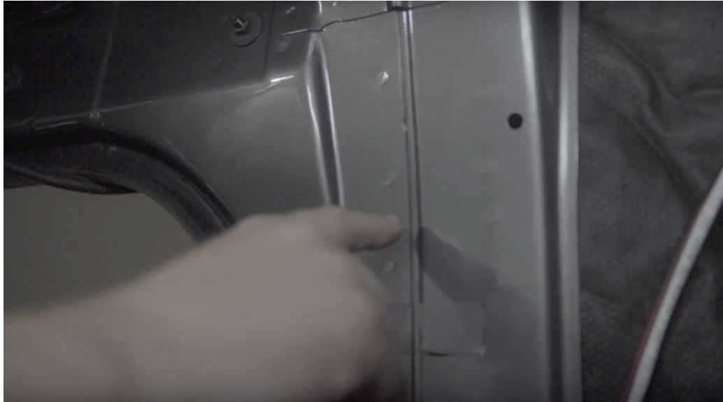
Centerline of van. Forward track mounts to the rear of this seam.
