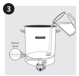
**Step 3** Slowly add filtered water to about 1 inch (2.5 centimeters) above the platform and filter. This is 3 gallons (or 11 liters) in a Pro Series 10 and 6 gallons (or 22 liters) in a Pro Series 20.
