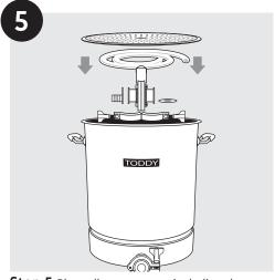
**Step 5** Place all components including the valve assembly, gasket, hose barb, hose, and tri-clamp into the bottom of the unit below the platform *to ensure they are fully submerged*. Clean with the valve in the open position.
