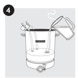
**Step 4** Add 2 to 3 liters of hot water to the brewer, then add Toddy® Cleaner per the chart below. *Allow the solution to fully dissolve*.
