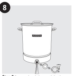
**Step 8** Remove the tri-clamp and cleaning blank over the sink, drain solution from the brewer, and allow all parts to air dry. (*Do not dry with a towel.*)
