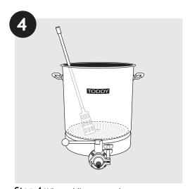
Step 4 When adding water, air may get trapped in the filter. If the filter bubbles up, gently guide the paddle across the platform toward the open end to push the air out, taking care not to tear the filter.
