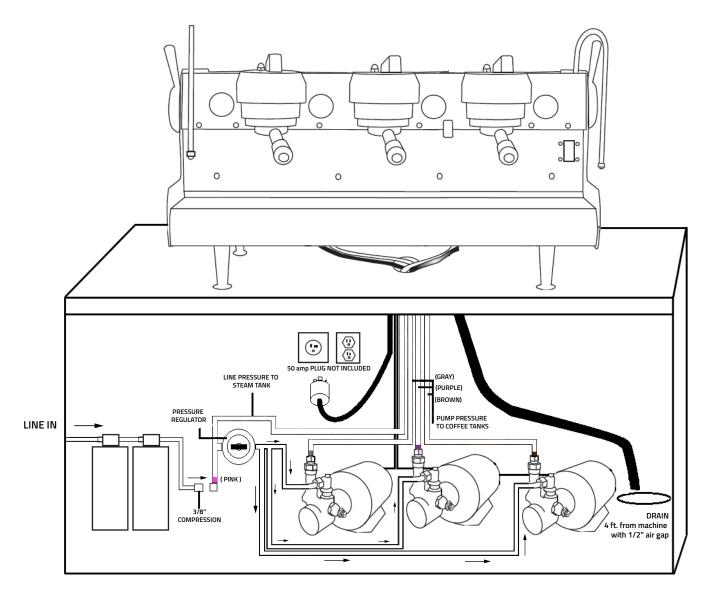
PINK =LINE IN FROM WATER FILTRATION TO THE STEAM TANK GRAY =LINE TO GROUP 1 (LEFT WHEN FACING MACHINE) PURPLE = LINE TO GROUP 2 (CENTER) BROWN = LINE TO GROUP 3 (RIGHT WHEN FACING MACHINE)
