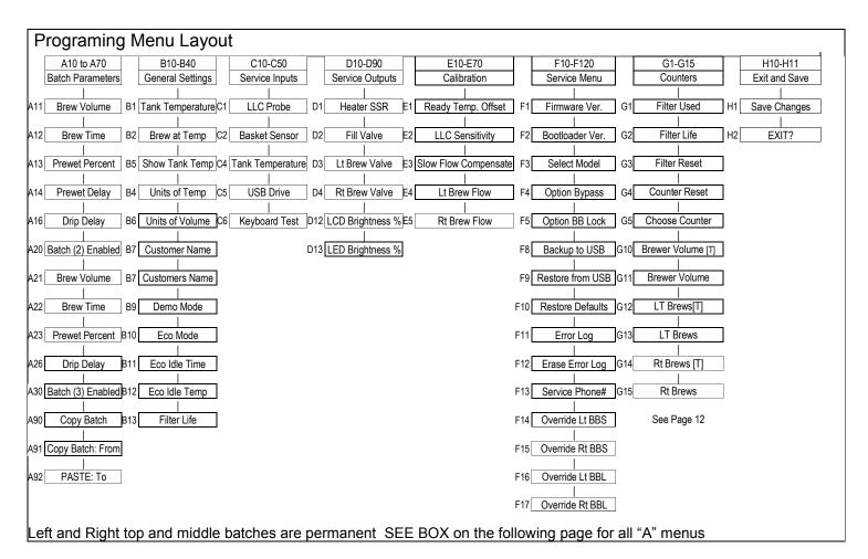
The "A" menu is the most accessed menu. It is for programming the batch volumes, brewing parameters, enabling or disabling brew buttons. The "A" menu moves through the six positions(CBS-1232+) or three positions(CBS-1231+) by entering the menu and pressing the left stop button. (only the left side is active for programming the CBS-1232+)
