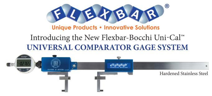
This highly versatile modular gaging system accommodates a wide range of internal and external measurements with ranges up to 40"/1000mm. The system's standard adjustable, spring loaded measuring beam with constant measuring pressure can accept a range of interchangeable measuring jaws, contacts and depth stops. Use with any 0-½"/12.5mm digital or dial indicator. Anvil travel range is 0.393"/10mm.
