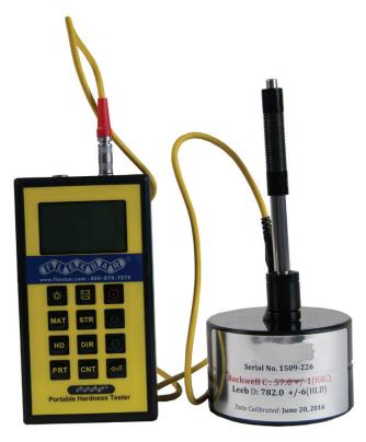
Note: Material thickness must be 1.5" or more for softer metals and 1" minimum thickness for steel.
