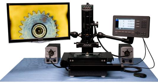
Offering exceptional value for the money, these systems offer highly flexible and upgradeable capacity. The MLX-2000 Series are compact and easy to use turnkey systems packed with powerful features including state-of-the-art color video, quality zoom optics and the MetLogix Mx200 Geometric Digital Readout
