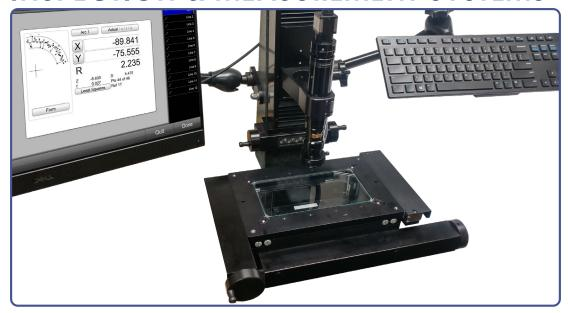
Opti-Flex MLX-3000 Series systems features a touchscreen monitor with geometric edge select tools. The powerful MetLogix M3 measuring software is intuitive and easy to use.
