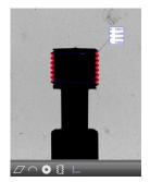
Also optional on request: M3 thread Inspection module: 18-M3-Thread
