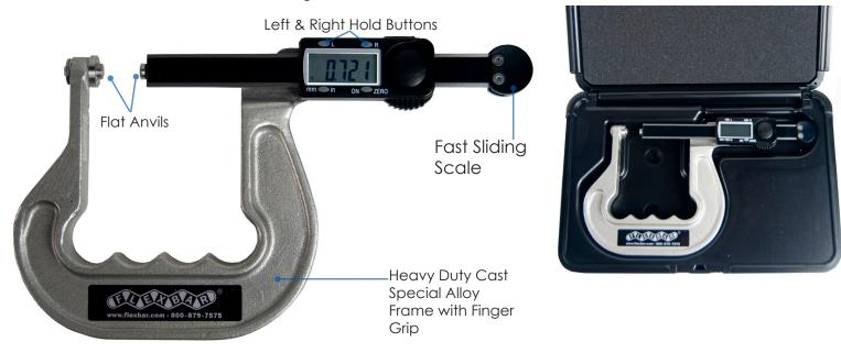
This rugged, yet lightweight micrometer provides quick and easy measurements for ranges up to 2.5"/63.5mm and will accommodate depths up to 3.3"/83.8mm. Ideal for shop requirements.
