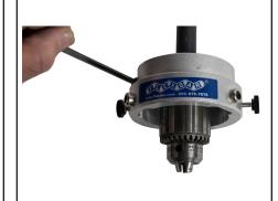
4. Install Clamp Assembly on Quill TIGHTEN CLAMP SCREW
