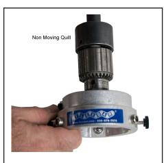
If your clamp and or bushing will not tighten sufficiently on Quill, please install shim.
