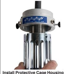
Install Protective Cage Housing Assembly. Slot lines up with Roll Pin.
