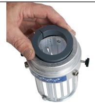
3. Install Optional Bushing if necessary. Line up slot openings. \*See Flexbar catalog or website for listing of available bushing adapters
