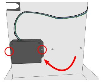
3. Rotate the controller box 180 degrees and secure it to the two studs using the two (2) 8-32 Keps nuts removed earlier. Make sure that the wires are routed as shown at left.
