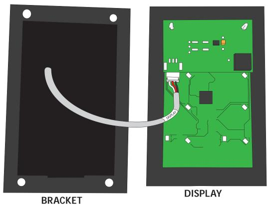
8. Place the display on the flush mount bracket as shown, attaching the back of the display panel to the magnets on the mounting bracket. Make sure that the alignment tab on the back of the display panel sits in the notch on the bottom of the bracket.
