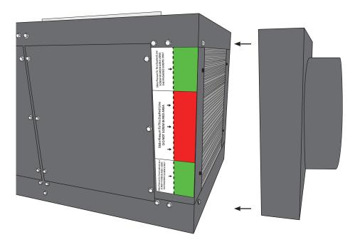
2. Drill two (2) screws through the plenum to secure it to the unit housing. Screws must be installed in the locations indicated on the red, green, and white installation sticker. Placing screws inside the red area will void the warranty.
