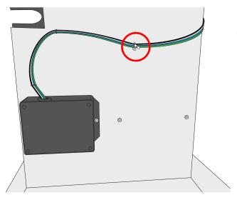
4. Resecure the wires using the twist clip.
