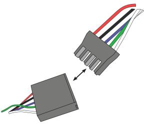
5. Remove the blower from its current location and connect the Molex connector. Ensure that the blower remains in the orientation shown.
