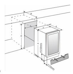
**NOTE:** When pushing the appliance into the niche, make sure that the main cable does not get trapped.
