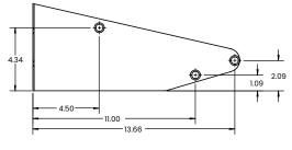
ROD POSITIONS, DISPLAY BRACKET 1 REMOVED FOR CLARITY
