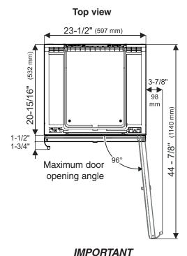
The floor on which the appliance stands must be horizontal and level. The kitchen units must be aligned horizontally and vertically.
