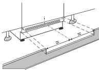
If the cabinets do not have a toe kick, a toe kick can be prepared and fitted just in front of the appliance.
