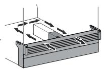
After installing the kitchen cabinet door, there must be a ventilation gap between the appliance ventilation grill and the kitchen cabinet door. The ventilation grille is movable to guarantee sufficient ventilation.
