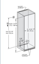
This is a fully integrated refrigerator-freezer appliance designed to be completely enclosed in a dedicated kitchen cabinet. This dedicated cabinet box must be constructed in accordance with the specified dimensions and must allow for sufficient air circulation to ensure proper operation. For more details about ventilation requirements, please refer to the Design Guide.
