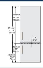
This is a door-on-door model, which means the custom panels are installed on the appliance doors.
