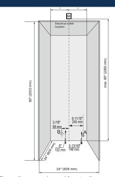
The appliances can be used freestanding or semi built-in. If semi built-in, consider the minimum cabinet opening dimensions specified on this image.
