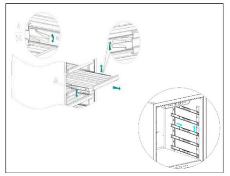
First remove all wine bottles from the shelf and pull it out as far as you can. Simultaneously press down the left lever onthe sliding shelf and press the right one up, pulling the shelf out at the same time. Next, push up on the shelf to release the front hook from the shelf bracket. Then just pull the shelf out.
