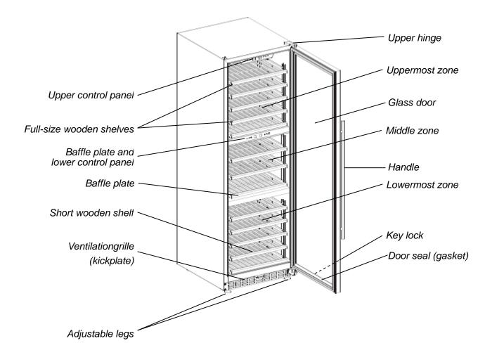
NOTE: Each zone has a Ventilation fan and a Sensor located on the rear wall.
