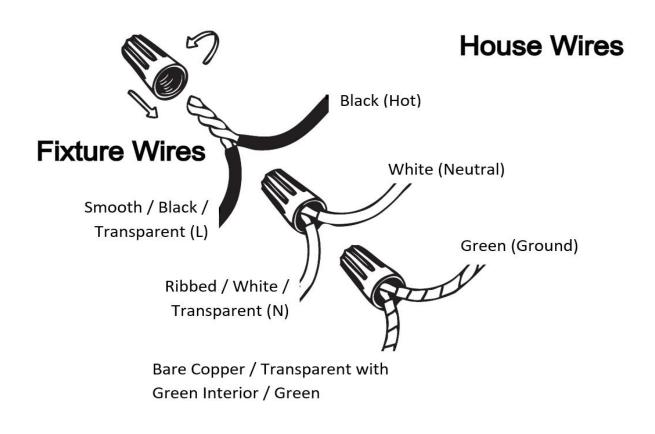
Use standard wire connectors to make all wire connections Twist connectors until wires are tightly joined Wrap each connection with approved electrical tape and carefully stuff all the connected wires into outlet box
