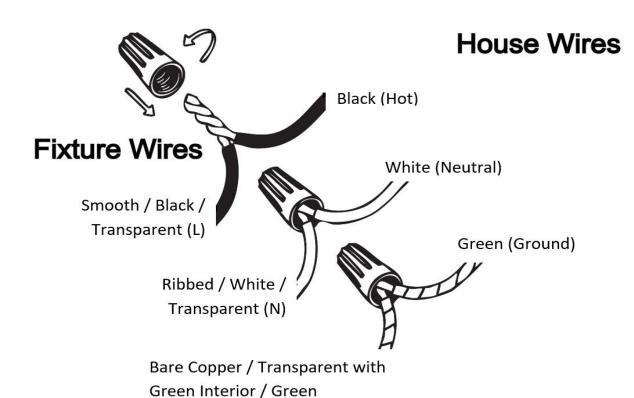
Use standard wire connectors to make all wire connections
