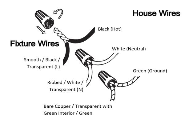
Use standard wire connectors to make all wire connections
