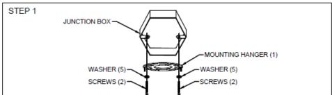
Secure the mounting hanger (1) to the electric junction box with the screws (2) and washers (5) provided.
