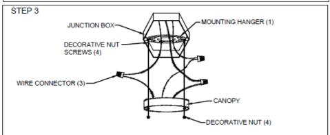
Install the recommended bulb in the socket, and then install the canopy (shade/cover) of the decorative fixture to the mounting hanger, using the supplied screws or decorative nuts (4).
