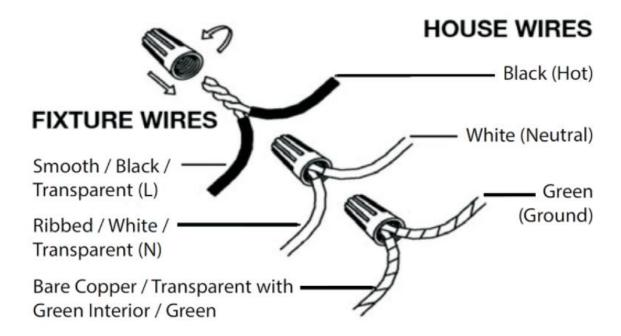
Use standard wire connectors to make all wire connections.
