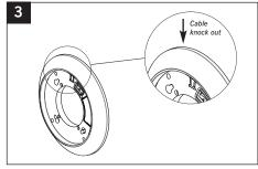
Remove cable knock out for the mains cable, ensuring sharp edges are removed to prevent damage to the cable insulation.
