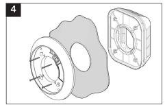
Secure window kit into position using the 4 screws provided within the loose item set. Screw lengths that can be used are:
