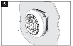
Secure back plate of the Unity CV2.1 / CV3 / CV3SV fan to the window kit using the shorter screws provided and wire as per the wiring section within the respective Unity Installation Instructions.
