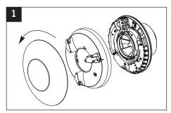
Rotate 'outer cover' anticlockwise until retaining clips are released and place the cover to one side. Loosen retaining screw in main body cover and rotate anticlockwise to remove.
