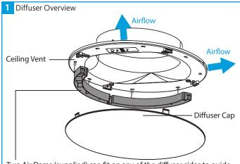
Two Air Dams (supplied) can fit on any of the diffuser sides to guide airflow away from a smoke detector and/or obstructions as required.
