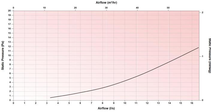
— Zehnder ComfoFit Therm insulated Flat 51 to Zehnder ComfoTube Therm insulated ø 90mm convertor
