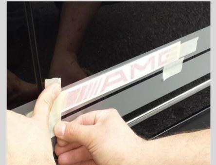
**Step 5:** Flip the graphic using the masking tape hinge so that it is face down on the surface and slowly peel the backing sheet away from the graphic.
