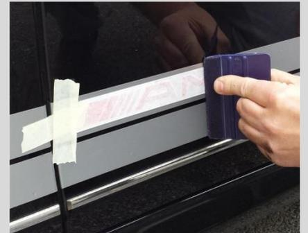
**Step 8:** Remove the low-tack application paper by pulling it back on itself at a 180° angle. Using this method to remove the application paper will reduce the chances of pulling the graphic back up and possibly causing air bubbles or edge lifting. Once you have removed the application paper, you may wish to go back and re-squeegee the graphic. Be careful not to scratch it.
