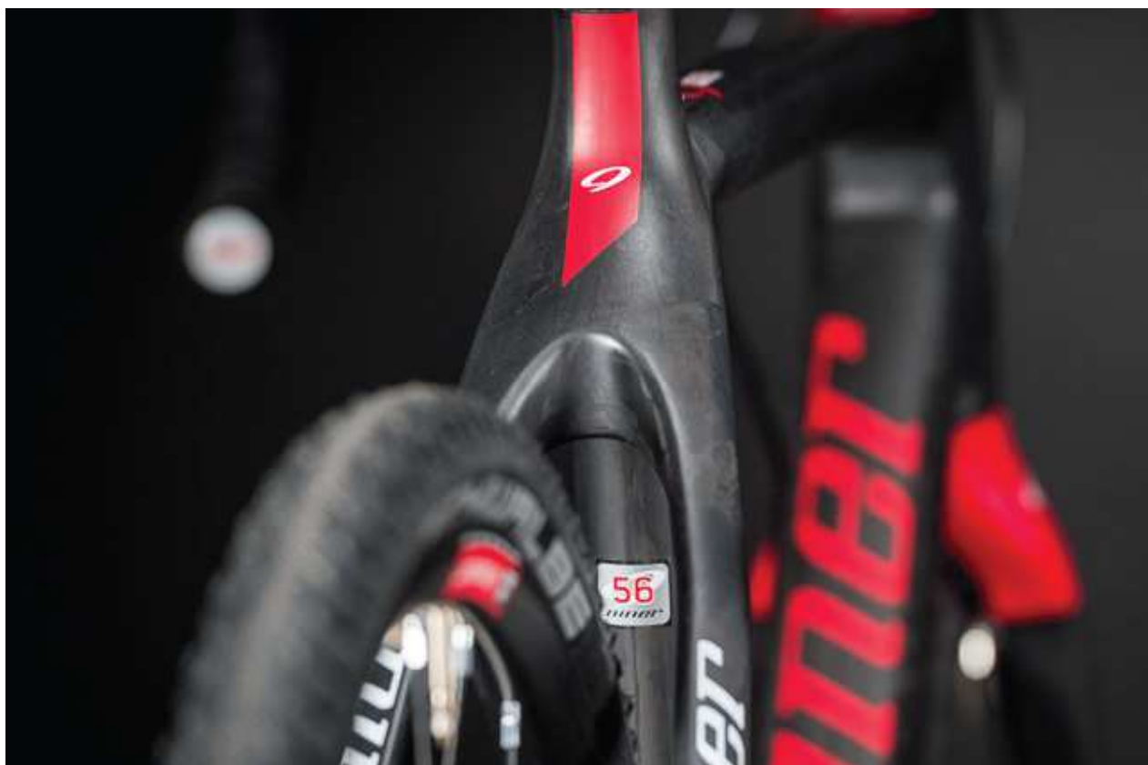
The BSB fork features a 15mm thru-axle. A new and trend sweeping the 700c world. Thru-axles provide a stiffer, more precise steering. Perfect for CX racing.
