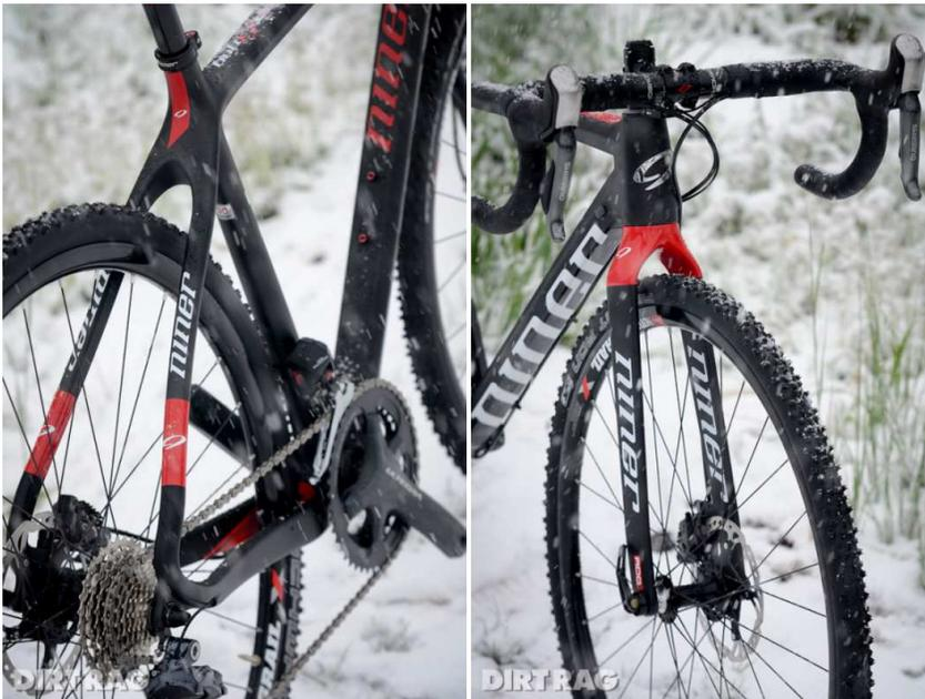
The PF30 bottom bracket provides a larger junction for the massive tubing and is compatible with the latest high-end cranksets. The disc-brakes are a natural choice as they provide superior stopping power in all conditions and additional mud clearance for the worst of days. While the fork uses a thru-axle, the rear end of the bike is a traditional 135mm quick release, to keep weight down.
