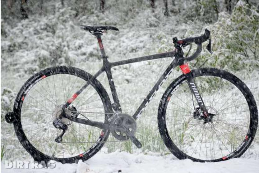
The frame is designed to be as stiff as possible when pedaling, so the downtube and chainstays are extra beefy, while the disc brakes mounted inboard allow for the seat stays and top tube to be specially tuned to provide a more compliant ride. It's paired with a 27.2 Niner RDO setback seatpost for maximum vibration and impact absorption.
