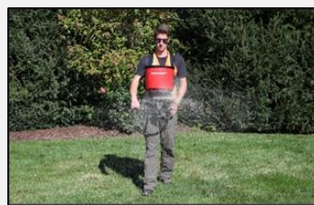
The 3-hole drop system allows for the spread to disperse in a 180
