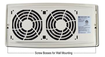
Drill out the bosses with a 3/16" drill bit and secure the HC500 to the wall. Directions are also provided on our instruction page.
