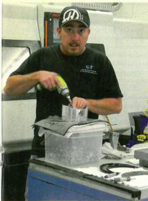
Employee Jason Carpenter is running a 6-axis machining center to precisely cut and then deburr a Lycoming piston.
