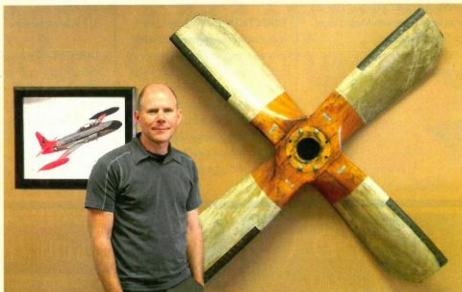
Mark Percario, owner of Combustion Technologies in Chatham, stands in front of a club prop used for test-running Pratt & Whitney radial engines.
