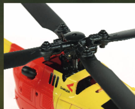
A ball raced main shaft and swashplate ensure the operational longevity of the robust composite rotor head.
