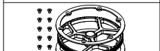
Main Pulley (x1) countersunk head hexagon socket screw M2x3mm (x12) Main Pulley Flanges (x2) Socket cap screw M2.5x15mm (x1) Nyloc Nut M2.5 (x1) Shim φ8xφ10x0.2mm (x1)
