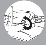
To loosen, or tighten, the brake handle use the supplied allen wrench to turn the nut on the other side of the collar. Setting of the handle should be firm. When set correctly the handle should rotate all the way to the collar and the speaker should not be able to rotate.
