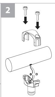
STEP 2. Connect or solder the wires from the clamp to the corresponding wires from your tower. Then loosely hand tighten the clamp bolts through the top half of the clamp around the tower and into the lower half of the clamp. Begin alternately tightening the bolts, with the supplied allen wrench, until both bolts are equally tight around the tower and the clamp is griping the tower bar.
