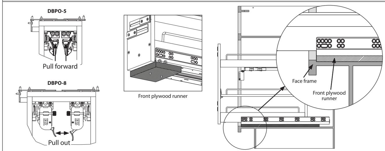
Remove the base from the unit by releasing the slide clips. In framed cabinets, center the unit in the opening making sure the front plywood runner is pulled tight against the back of the face frame. For frameless cabinets, place the unit within 1-1/2" of the left of the cabinet and the front plywood runner needs to be set back 3/4". Install with the four (4) #10 x 3/4" Pan Head Wood Screws provided in the four pre-drilled holes in the runners.
