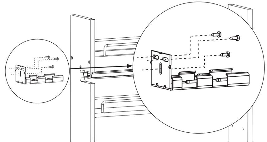
Remove the unit from the base again and then slide the rear mounting bracket off the slide. Align the rear bracket prongs with the indentation marks on the rear of the cabinet and secure with three (3) #8 x 5/8" Pan Head Wood Screws in the slots as shown. Re-install the unit onto the slides, making sure as you push it in the cabinet, that the top slide is properly seated into the rear mounting bracket. Operate the unit to make sure the undermount slides are working properly.
