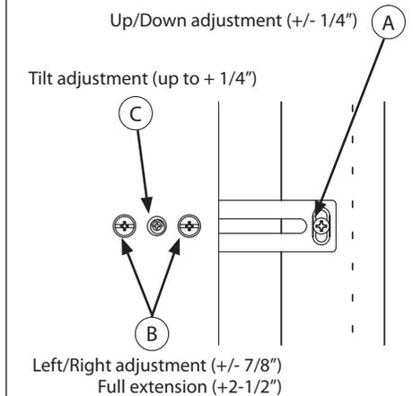
To adjust door up or down loosen door mounting screws (A). To adjust left or right, loosen both set screws (B) adjust and retighten. To adjust tilt, loosen both set screws (B) and then turn tilt screw (C) clockwise to desired distance and then retighten set screws.
