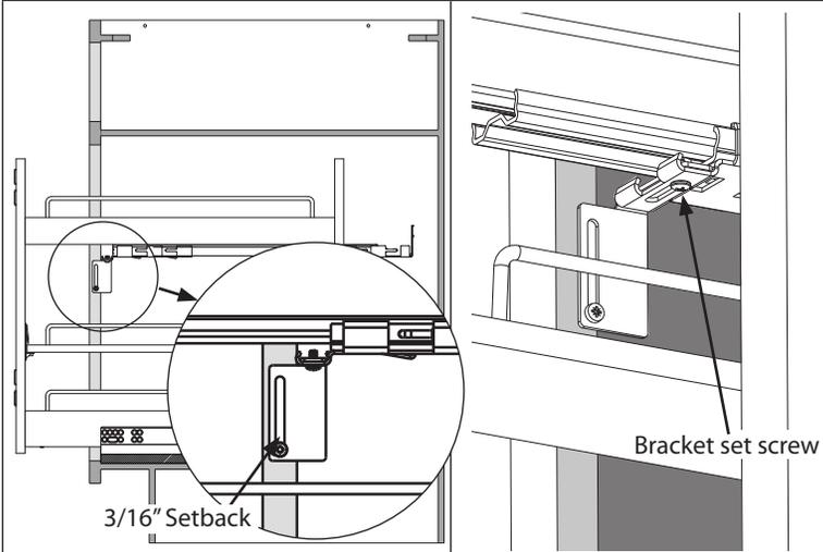
Pull the top front mounting bracket into position on the side of the face frame (or cabinet) allowing for a 3/16" setback (shown left above). Firmly secure with one (1) #8 x 5/8" Pan Head Wood Screw. Make sure the gap between the unit and the side of the face frame is equal from top to bottom. Adjust accordingly and then securely tighten the bracket set screw (shown right above). Operate the unit and make adjustments as necessary for the slides to operate smoothly.
