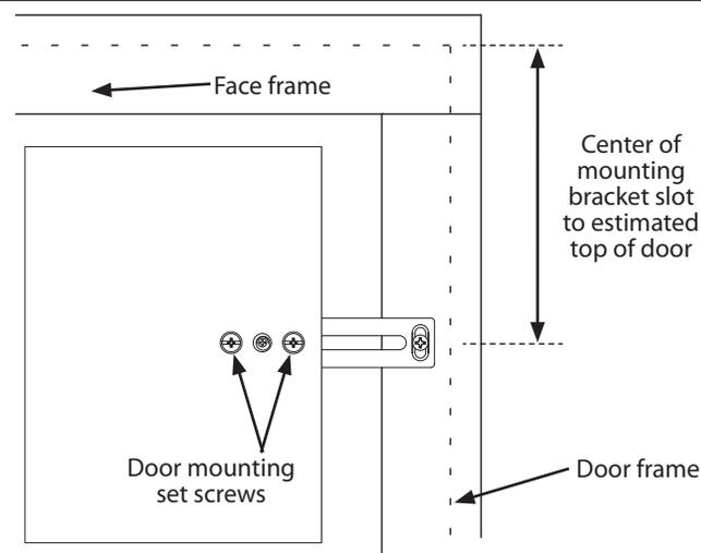
Loosen the door mounting set screws and slide bracket out to desired position to attach to the door rail. Measure from the center of the slot on the door mounting bracket to the estimated top of door. Mark door with measurement for both top brackets. Install door with the four (4) #8 x 5/8 Flat Head Phillips Wood Screws provided. (NOTE: DETERMINE CORRECT SCREW LENGTH TO DOOR PANEL THICKNESS)
