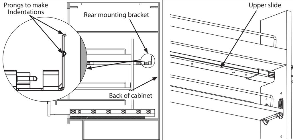
If the countertop is installed, pull the organizer partially open to gain access to the upper slide. Firmly grasping the upper slide, tap it against the back of the cabinet. The rear bracket should make small indentations in the back of the cabinet. Proceed to step 3. If countertop is not installed, remove top drawer and pull the organizer partially out to gain access to the rear bracket. Install three (3) #8 x 5/8" Pan Head Wood Screws provided in the slots. Proceed to step 4.
