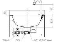
Suggested mounting height from floor level for standard use - 850mm-900mm
