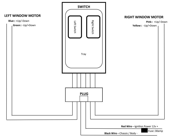
(ATT:: When fitting to Holden Commodore, connect the Red power wire to thick Pink wire at Commodore Key Wiring)
