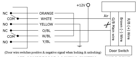
AIR COMPRESSOR LOCKING SYSTEM eg: AUDI-BENZ
