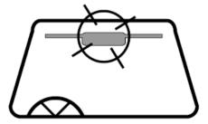
3 Remove the protection film from the antenna.
