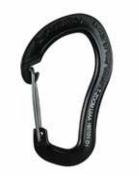
A wire gate carabiner uses a loop of stainless steel wire as the gate. Although it appears as though it might not be as strong as the straight gate or bent gate, it is. The wire itself creates a "spring to close" gate, eliminating the need for an extra mechanism and making the carabiner very lightweight. In addition, there is no spring mechanism so the gate will never freeze shut.
